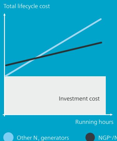
With an air factor\* of 1.8 (at 95%) to 5.5 (at 99.999%) and a special cycle time modulation algorithm, the running cost of the new NGP<sup>+</sup> can be reduced by 50%, compared to other N<sub>2</sub> generators.
